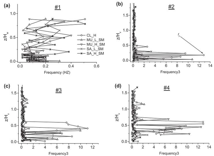
Fig. 6. The Fast Fourier transform of instantaneous velocity. Completely submerged vegetation of (a) profile #1 depicted in Fig. 1; (b) profile #2; (c) profile #3; (d) profile #4.
