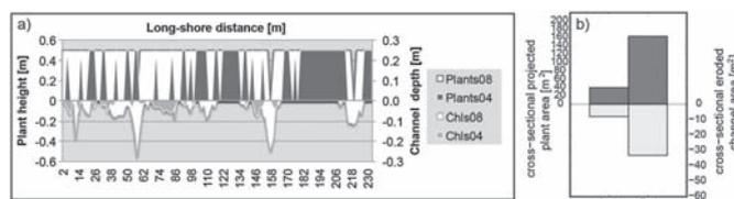
Fig. 9. (a) Long-shore profile at Walsjoorden in 2004 and 2008 at its maximum erosion zone (see also white line Figure 7). (b) A comparison between the cross-sectional projected plant area (dark gray) and the cross-sectional eroded channel area (light gray) along the long shore profile at this two time points (2004 and 2008).
