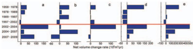
Fig. 4. Net volume changes between erosion and accretion during different intervals: a: the region above the -10 m isobath between the N. Channel and N. Passage; b: the region above the -10 m isobath between the N. and S. Passages; c: the region of the Nanhui Shoal and S. Passage above the -10 m isobath; d: the seaward region below the -10 m isobath; e: the entire submerged delta; The red line shows the demarcation between the pre-TGD and post-TGD eras.
