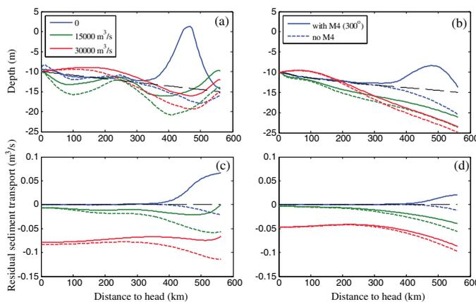
Fig. 8. (a,b) Bed profiles after 4000 morphodynamic years and (c,d) tidal residual sediment transport over 4000 years in the convergent basin as shown in Figures 8a and 8c and in the rectangular basin as shown in Figures 8b and 8d. The black dashed lines indicate the initial bed profiles in Figures 8a and 8b and indicate the zero level in Figures 8c and 8d.
